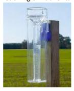
Keep a **rain gauge** in your garden (a good Christmas present), check the gauge regularly, this way the exact amount can be recorded; you can regulate your watering accordingly. A reading of 40mm on the gauge equals approximately 15 litres.
